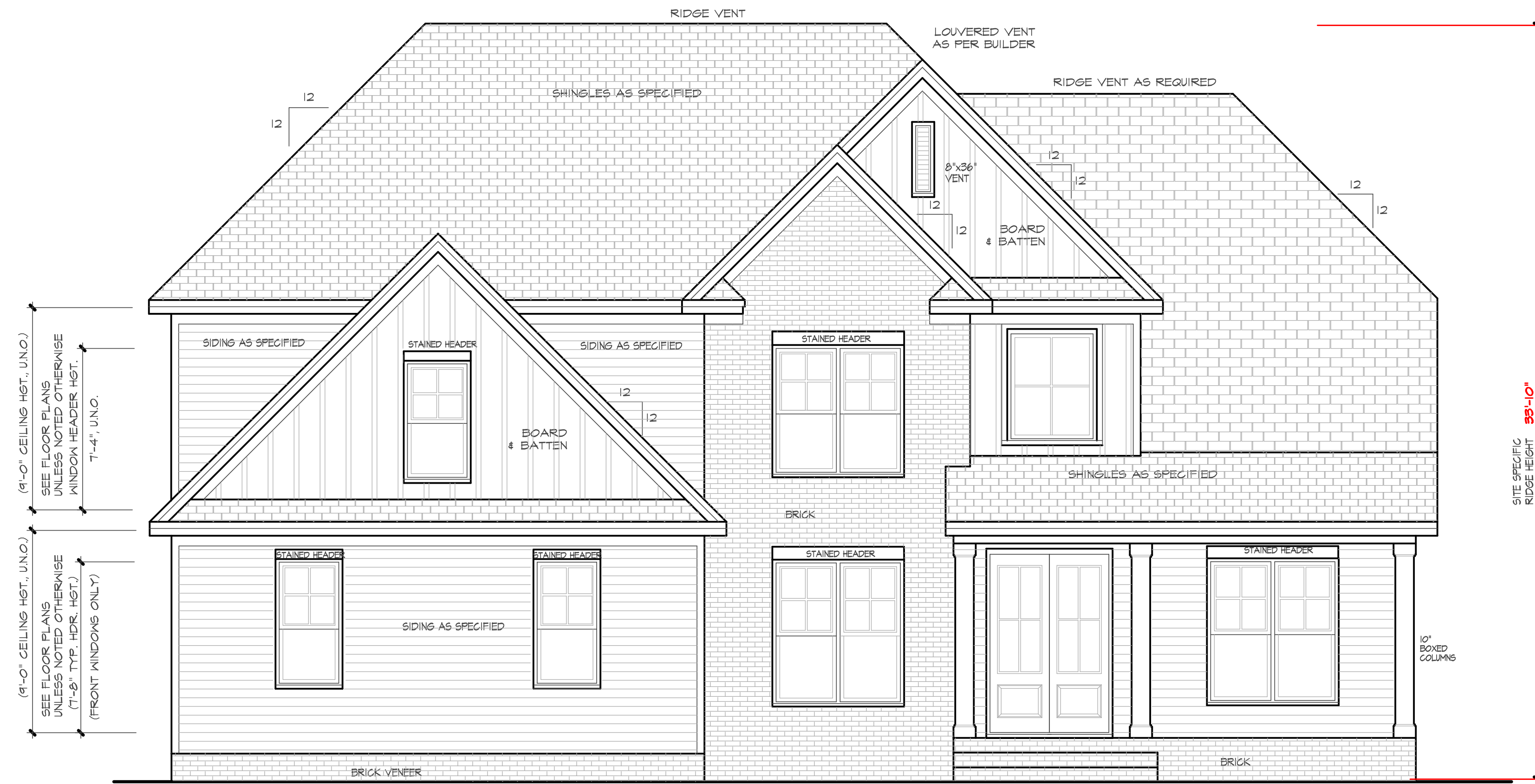
FRONT ELEVATION SCALE 1/4" = 1'-0"
